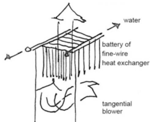
Figure 1: water/air Fiwihex heating/cooling
