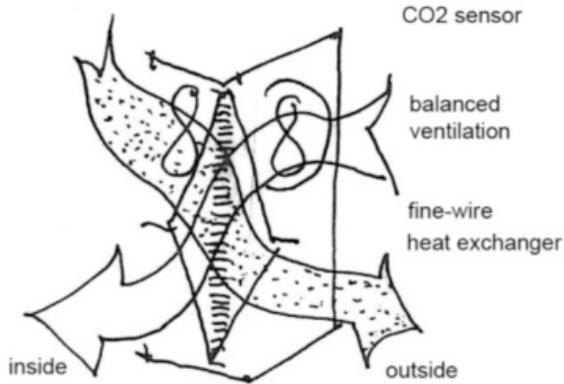
Figure 2: air/air Fiwihex balance ventilation
