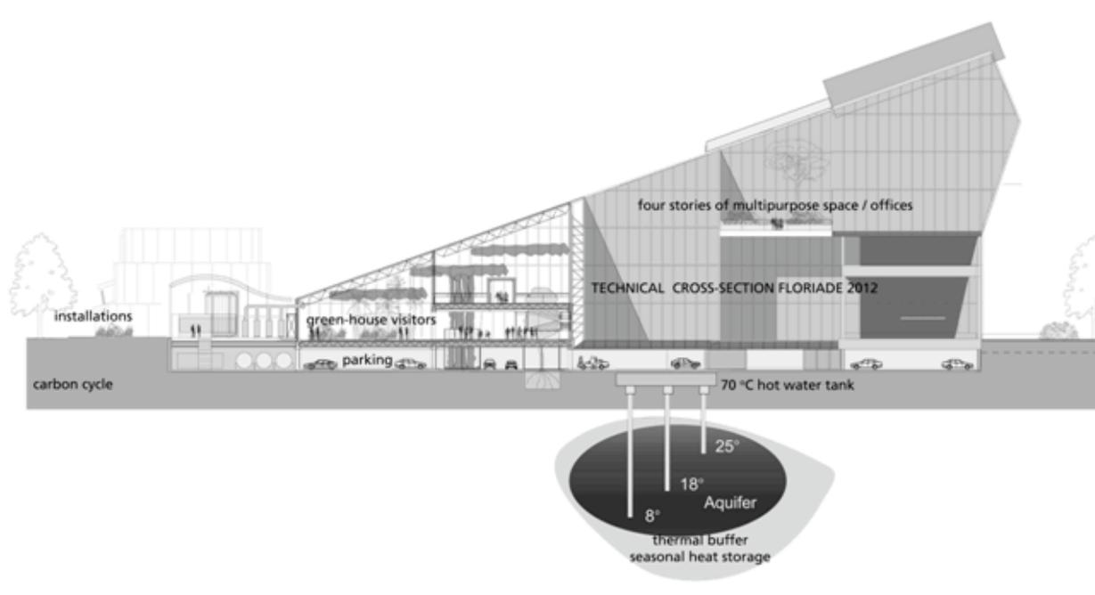
Figure 7: East façade cross section - Floriade 2012 world exhibition glasshouse - integrated design of 40.000 m<sup>2</sup> with an anaerobic waste treatment and seasonal heat and cold storage in wet sand
