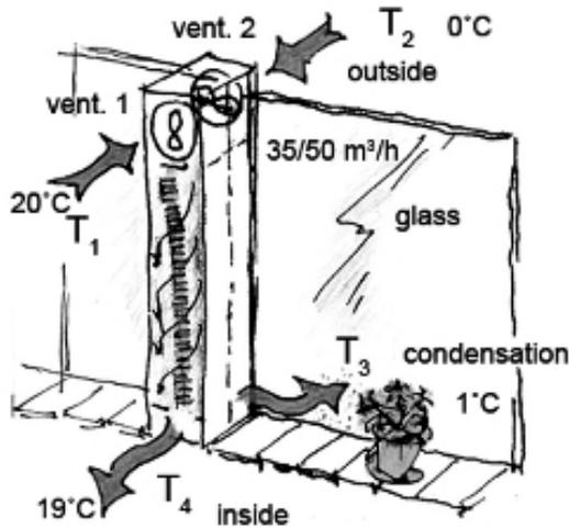
Figure 8: Operation scheme of a Breathing Window
