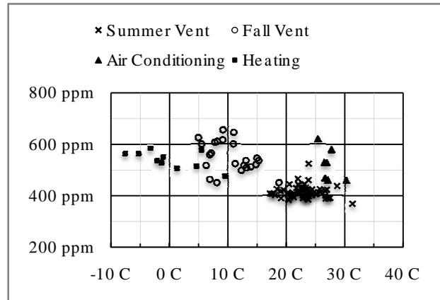
Figure 4: Average daily UEC office CO<sub>2</sub> concentration as a function of average daily outdoor air temperature for heating, cooling and natural ventilation.
