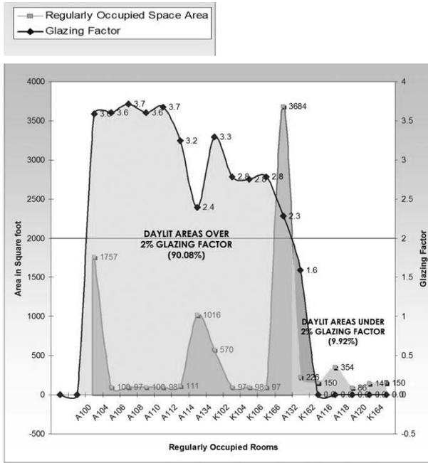
Figure 4.4: Chart showing comparison of Daylit regularly occupied spaces in the Porterville Main Kitchen Design with the non-Daylit ones
