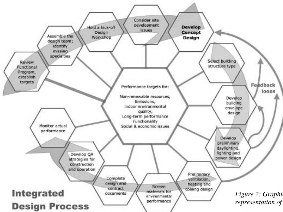
Figure 2: Graphical representation of the IDP process.
