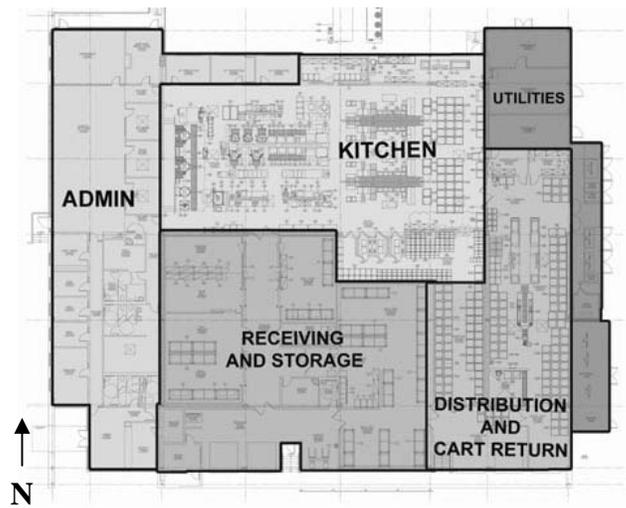
Figure 4.3: Functional and Circulation plan for Napa Main Kitchen
