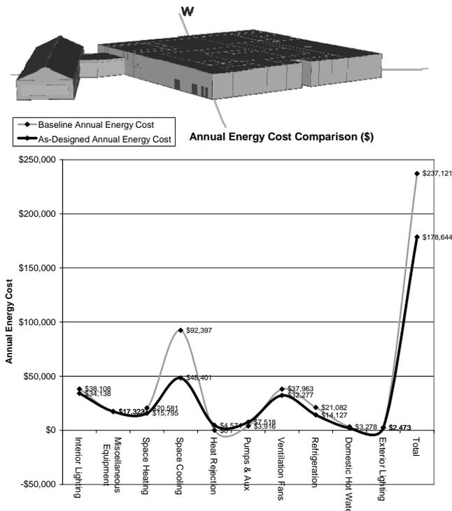
Figure 5: E-quest energy model for the Porterville Kitchen (Top) and the Annual Energy Cost Comparison chart (Bottom). The Design case provides up to 24.7% in energy cost savings over the base case scenario.
