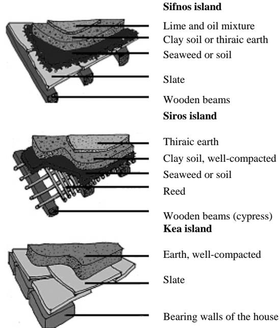
Figure 2: Sections of typical flat roof construction in islands of the Cyclades complex.
