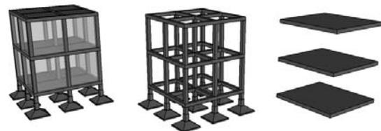
Figure 1: Default Building (left) fixed columns, beams, foundations, and Slabs (middle and right)
