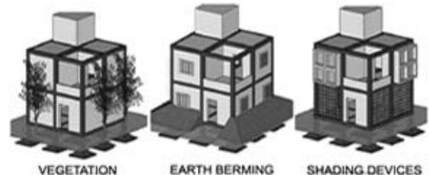
Figure 8: Multiple ways to avoid heat gain due to solar radiation
