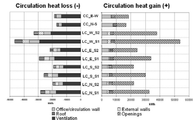
Figure 3: Circulation heat gains and losses.
