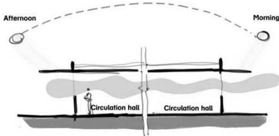
Figure 4: Partial shading of central circulation openings.
