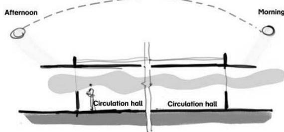
Figure 4: Partial shading of central circulation openings.
