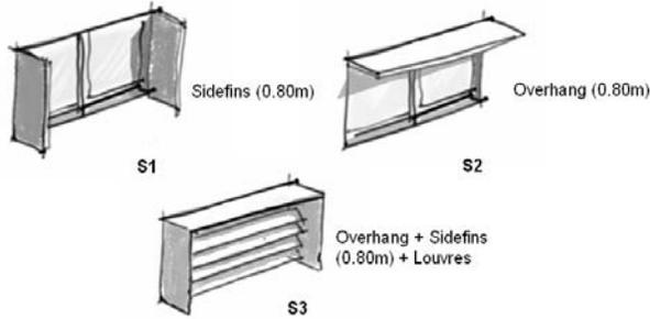
Figure 7: Simulated shading devices.
