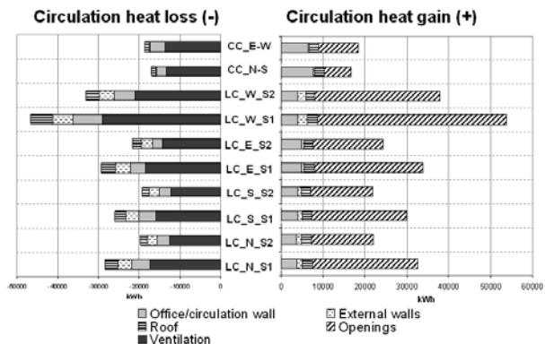
Figure 3: Circulation heat gains and losses.
