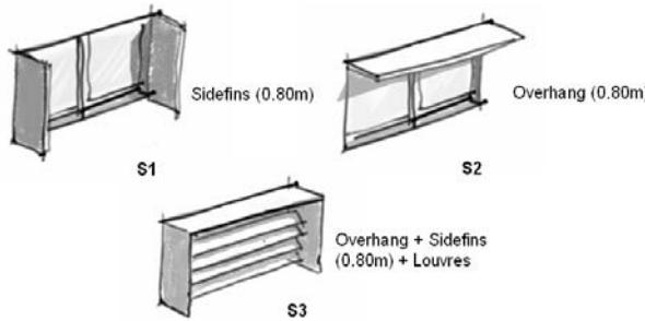
Figure 7: Simulated shading devices.
