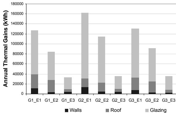
Figure 2 :Annual thermal gains of simulated cases..
