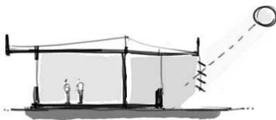
Figure 5: Shading device of a West oriented circulation hall.
