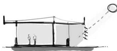
Figure 5: Shading device of a West oriented circulation hall.
