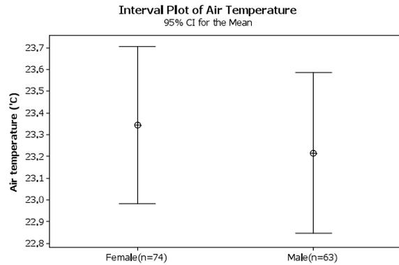
Figure 4: Thermal conditions in female and male groups (average 23.34°C (female) vs. 23.22°C (male),  $p=0.62$ ).
