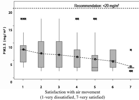
Figure 10: Correlation between air movement satisfaction and particulate levels in workstations ( $n=133$ ,  $R=-0.255$ ,  $p=0.003$ )
