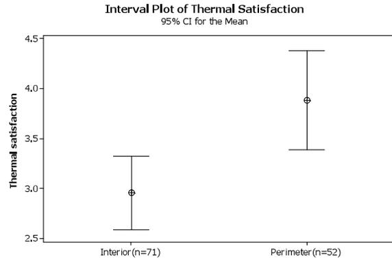
Figure 2: Confidence Interval comparison of occupant thermal satisfaction level between perimeter and interior zones with cooling season data (average 2.96 (Interior) vs. 3.89 (Perimeter), p=0.003).
