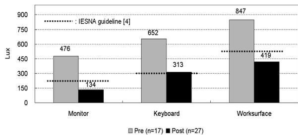
Figure 6: Comparison of illuminance between Pre and Post conditions and IESNA guideline (all comparison sets are statistically significant with  $p=0.000$ ).
