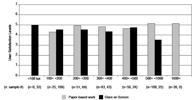
Figure 8: Changing patterns of user satisfactions with lighting level on workstation surface for paper-based work and glare on computer monitor screen (The satisfaction scores follow the scale in Table 1).
