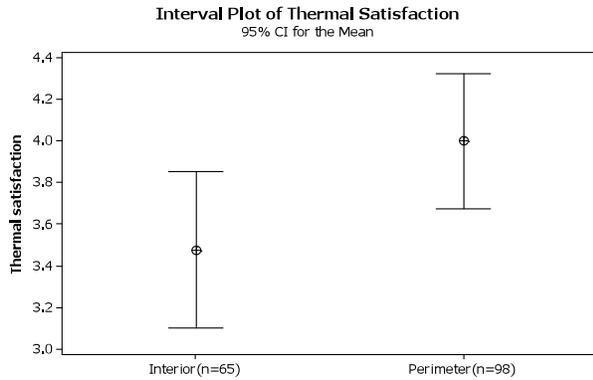
Figure 3: Confidence Internal comparison of occupant thermal satisfaction level between perimeter and interior zones with heating season data (average 3.48 (Interior) vs. 4.00 (Perimeter),  $p=0.04$ ).
