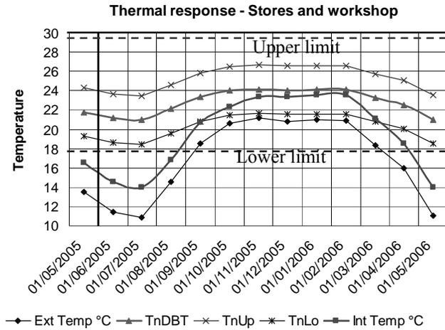
Figure 4: showing the thermal response of the stores and workshop to changes in exterior temperature on a month by month basis from May 2005 to May 2006.
