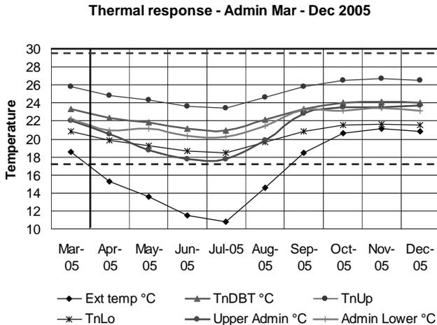
Figure 2: showing the thermal response of the administration block to changes in exterior temperature on a month by month basis from March 2005 to December 2005
