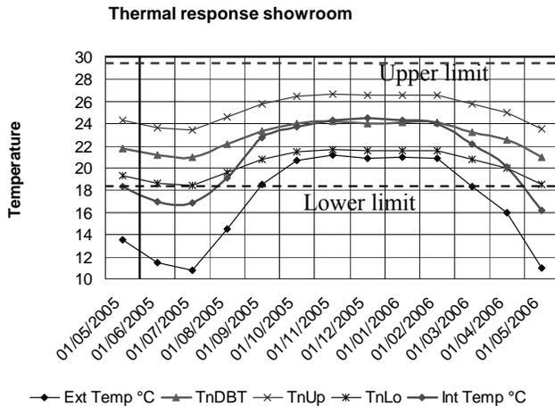
Figure 3: showing the thermal response of the showroom to changes in exterior temperature on a month by month basis from May 2005 to May 2006.
