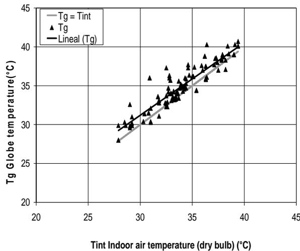
Figure 7: Air temperature vs. globe temperature indoors during the summer survey period (black triangles and black line). Gray line is  $T_g = T_{int}$
