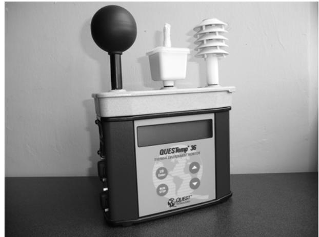
Figure 6: Thermal environmental monitor
