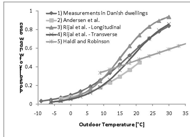
Figure 1: The probability of open window as a function of the outdoor temperature. The curves are a result of logistical regression
