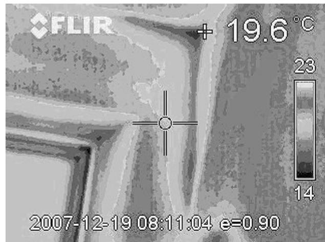
Figure 4: Thermal image of external corner of east bedroom, first floor; the dark areas show cold internal corners,
