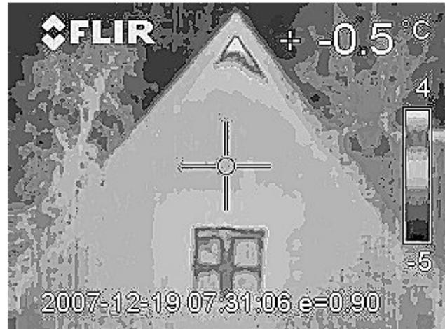
Figure 3: Thermal image of stone clad gable, the light areas show areas of significant heat loss at apex of roof
