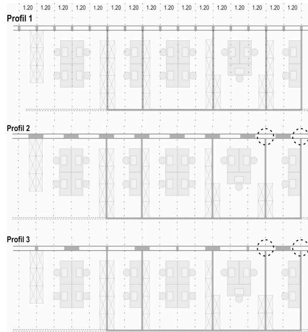
Figure 1: Confrontation of an irregular space division (full flexibility test) with 3 facade designs: fully glazed, window's array based (1 for every 2 axis) and window's array based (1 every 3 axis). For designs based on window's array, local discomfort occurs (dotted circles).
