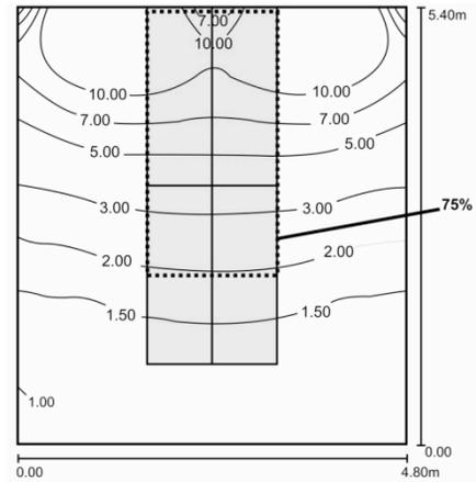
Figure 4: daylight factor levels for the “aware flexibility – level one” concept shown in Fig.3 and a 40% glazed facade. The dotted line identifies the 75% of spaces occupied for critical visual tasks.
