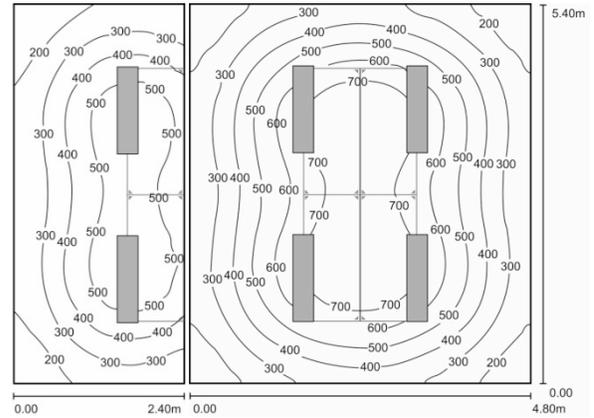
Figure 5: Dialux simulation of the artificial lighting in an aware flexibility concept – level one. Lighting devices simulated are Zumtobel L-FIELDS A A 2/28W. Resultant power is 9.46 W/m<sup>2</sup>.
