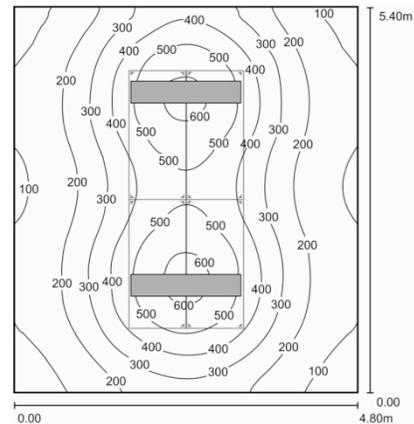
Figure 6: Dialux simulation of the artificial lighting in an aware flexibility concept – level two. Lighting devices simulated are Zumtobel L-FIELDS A A 2/35W T16. Resultat power is 5.83 W/m<sup>2</sup>.
