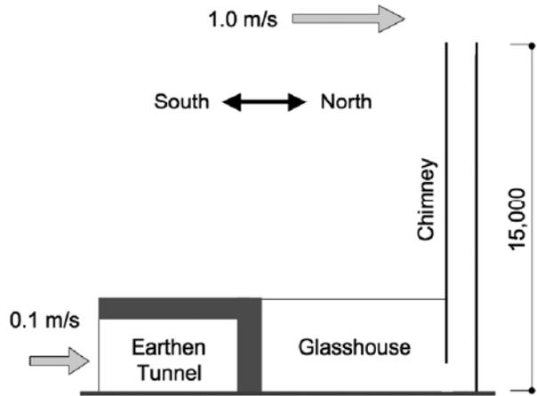
Figure 4: Given Conditions of Wind Velocity and Direction.
