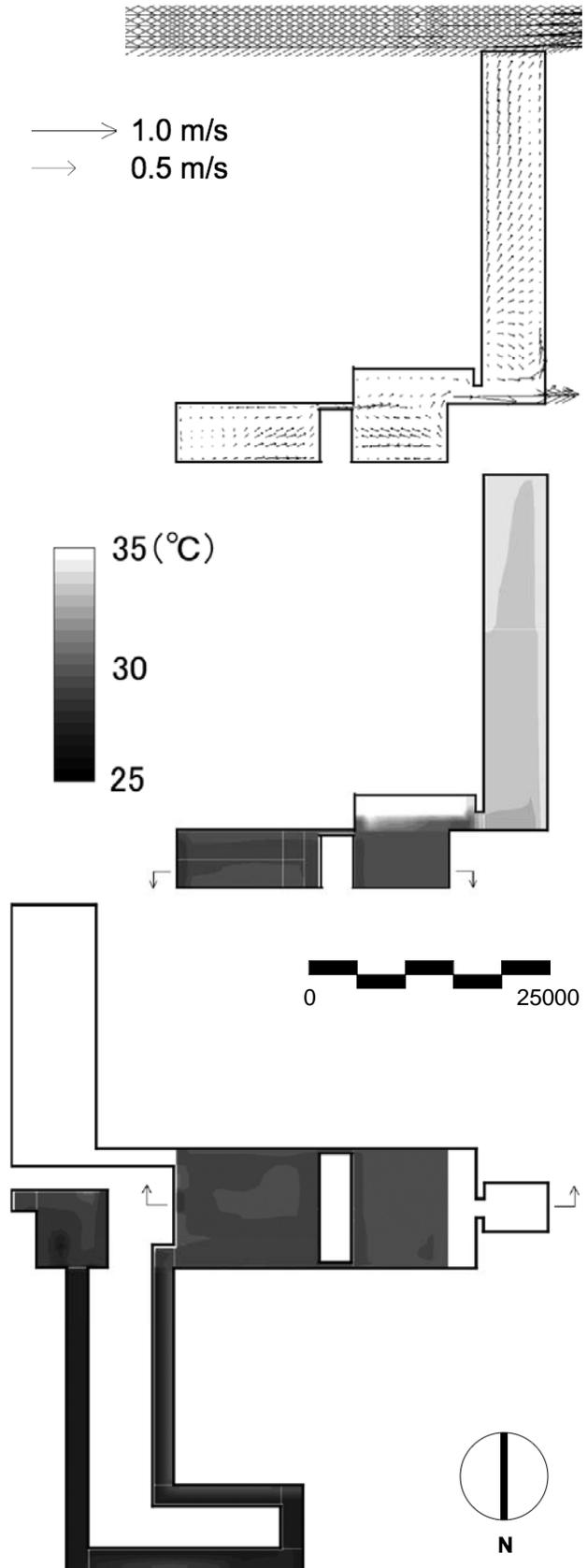
Figure 11: Wind Velocity and Air Temperature Distribution. (Calculation Result, 1300, August 10, Standardized Year)
