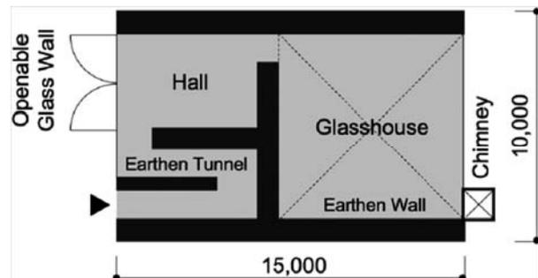
Figure 2: Building Model Plan of Public Space with Abandoned Chimney Reused as a Solar Chimney.
