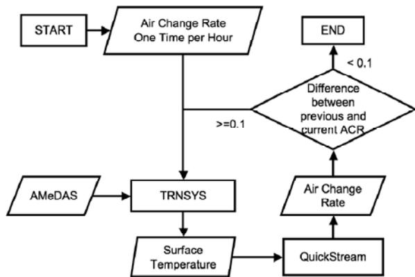
Figure 3: Calculation Flow of Each Time Step.
