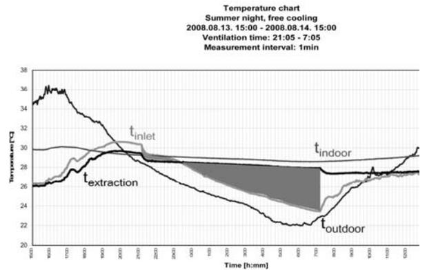
Figure 4: Summer night operation mode, free cooling (the highlighted area indicates useful cooling)
