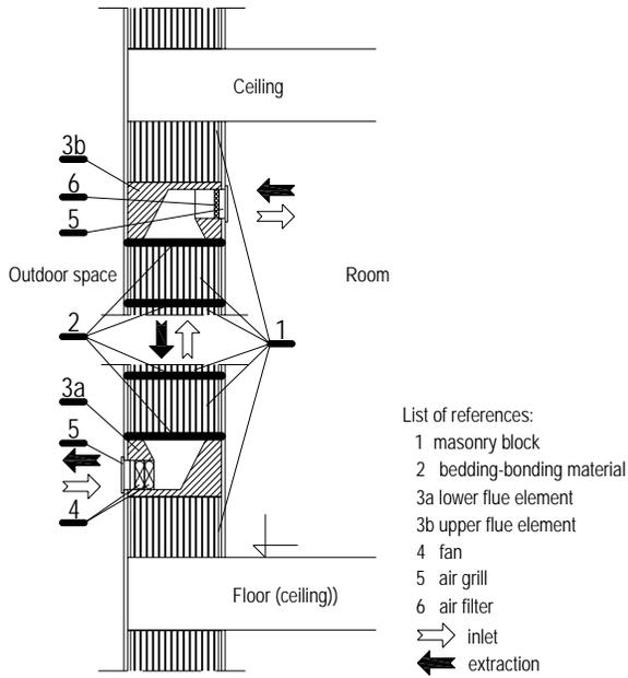
Figure 1: Schema of the ventilation system
