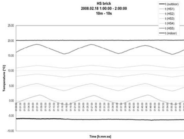
Figure 2: Variation of typical temperature values (Example 2, alternating interval: 10 minutes, the increasing values indicate measurements upward from the bottom of the flue by 50 cm intervals)
