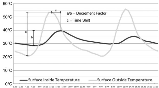
Figure 10: Example of the calculation of time shift and decrement factor of the reference envelope system.
