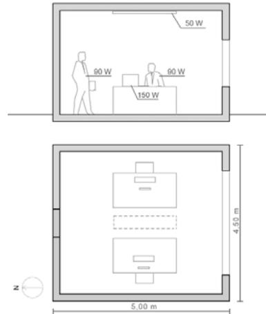
Figure 8: Section and floor plan of the virtual test-room.
