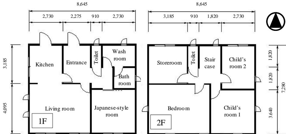
Figure 3: Floor plan of a standard residential house model proposed by the Architectural Institute of Japan
