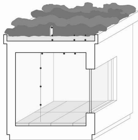
Figure 4: Green roof data logger locations
