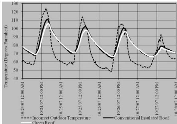
Figure 5: Interior temperatures at 20" from the floor for October 24 to 27
