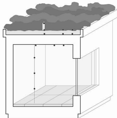
Figure 4: Green roof data logger locations
