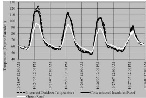
Figure 6: Roof surface temperatures at 24" from the edge for October 24 to 27
