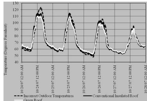
Figure 7: Temperatures 4" above the roof surfaces
