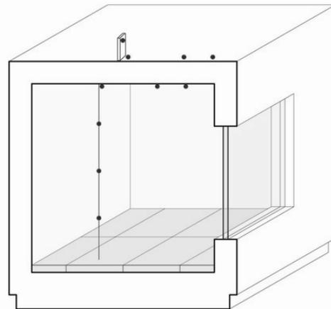
Figure 3: Conventional insulated roof data logger locations
