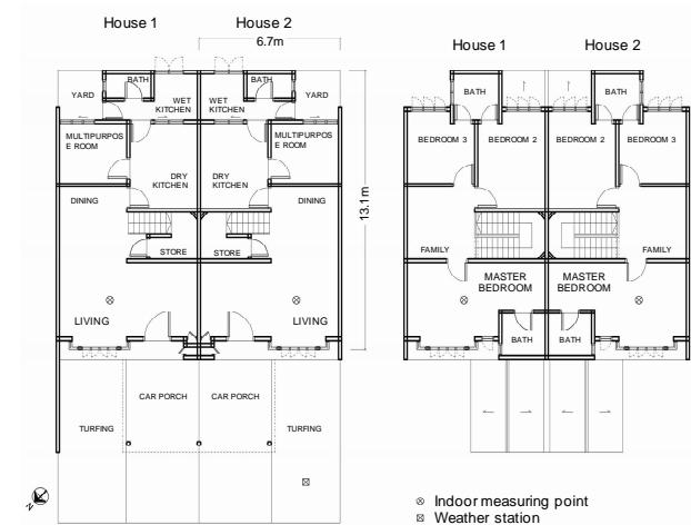
Figure 2: Floor plans of the case study houses.
