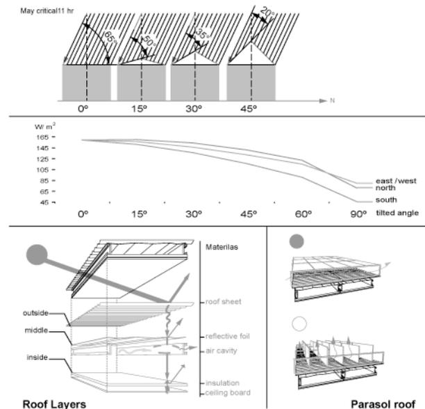
Figure 4: The roof: tilt angles vs. solar radiation, layers and parasol.
