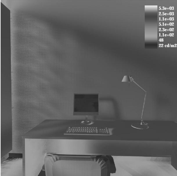
Figure 3a. Falsecolour luminance map ( $\text{cd/m}^2$ ) rendered with the BSDF data. Mirror-VB, December 21, at 9:00 AM.
