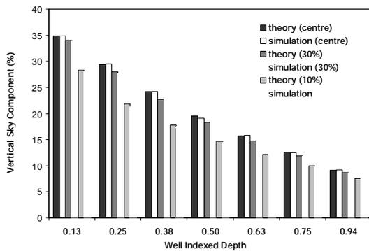
Figure 3: Vertical Sky Component comparisons between theoretical calculation and Radiance simulation.
