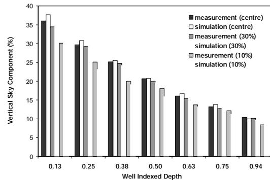
*Figure 2: Vertical Sky Component comparisons between measurement and Radiance simulation.*
