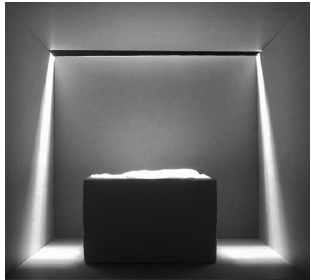
Figure 3. Photography of the physical model (plaster block linear aperture, direct source of light).
