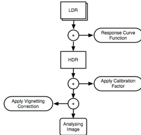
Figure 4: A systematic diagram showing essential steps for calibrating HDR image.
