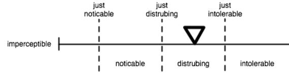
Figure 2: Scale proposed by Osterhaus et al. [9] describing the degree of discomfort glare perceived by subjects.
