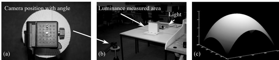
Figure 5: Equipment setup for estimating the vignetting function (a) and (b), and estimation result (c) for correcting the vignetting effect of the images.
