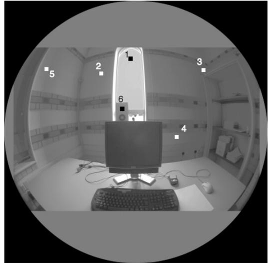
Figure 7: A field-of-view image showing the scene of the experiment and patch locations for luminance assessment.
