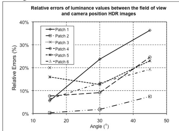
Figure 8: The effect of the camera position dependent on the deviation of the angle.
