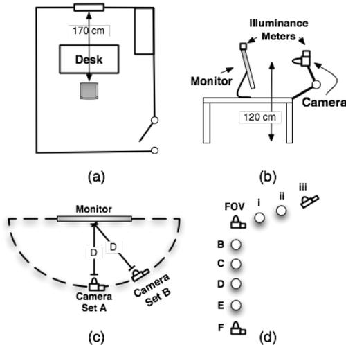
Figure 6: Experiment setup in controlled office block: (a) floor plan view; (b) side view of subject's work desk; (c) camera pairs setup; and (d) Angles and distance parameters layout.
