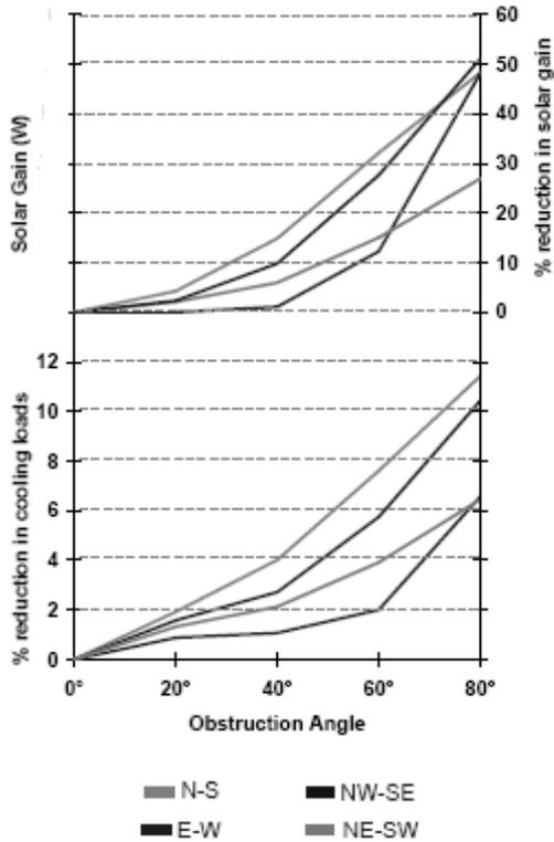
Figure 4: Effect of street canyon and street orientation on internal cooling loads. [4]
