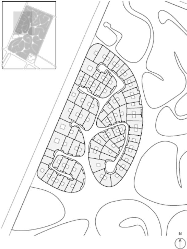
Figure 9: Detailed Plan of a section of the proposal showing the plot divisions, plot entrances and courtyards
