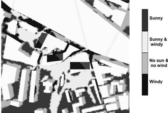
Figure 4: Illustration of sunny/windiness around the proposed development in June at 3pm.
