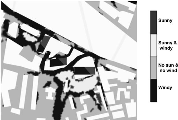
Figure 5: Illustration of sunny/windiness around the proposed development in December at 3pm.
