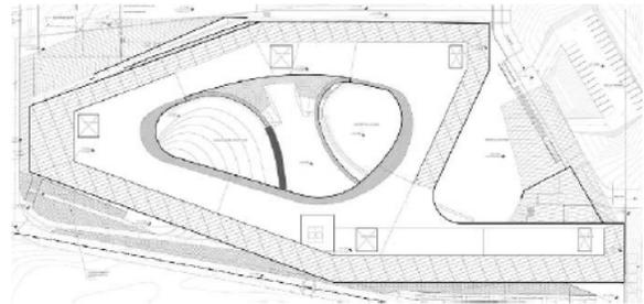
Figure 6: Building layout illustrating the inner core zones, atria locations, bar-sections and perimeter zones
