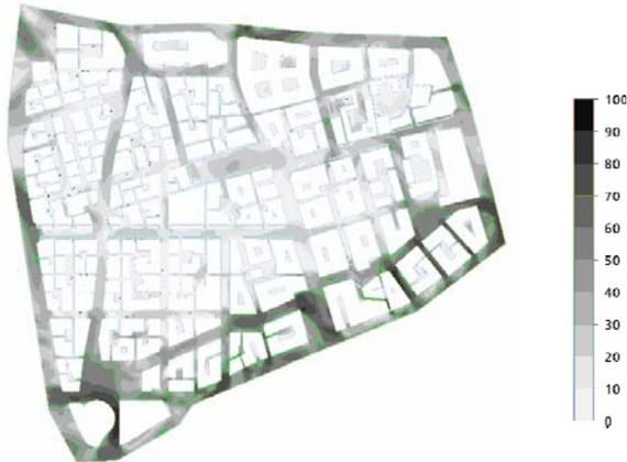
Figure 3: Percentage of exceedence for a wind speed greater than 2m/s (400fpm)
