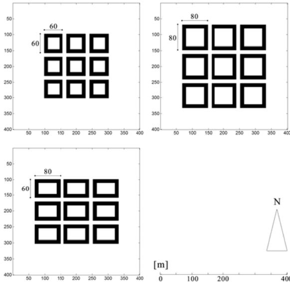
Figure 1: The analysis investigates 6 urban blocks configurations. Above the 3 basic layouts that were also analysed with a rotation of 45°. Blocks are 12 meters high.
