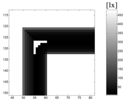
Figure 3: Detail of one building showing the estimated illuminances (lux) distributed indoors on the 15<sup>th</sup> of April at 5 PM. Note the non-passive zones in the middle of the corner.
