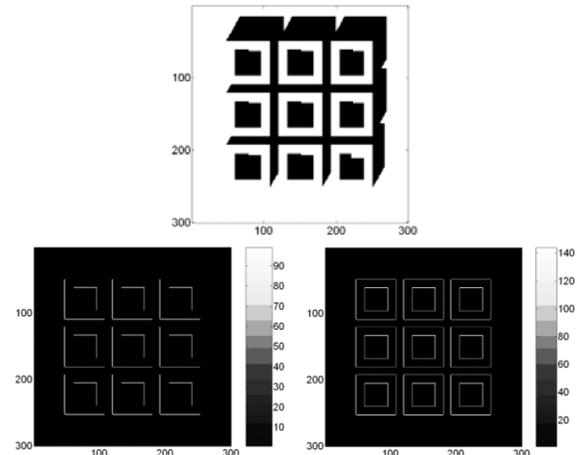
Figure 2: On the top: (a) Shadows' map. Bottom left, (b) percentage of direct solar radiation and right (c) collected on each facade on 10 December at 2PM ( $W/m^2$ ).
