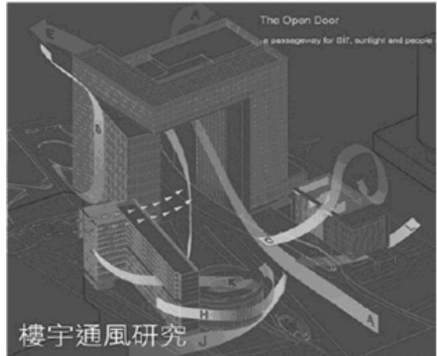
Figure 8: A visualisation of wind flow around the proposed building. (Courtesy Rocco Design Architects Ltd.)
