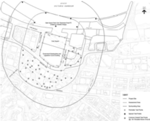
Figure 6: Test point distribution map of the AVA Detail Studies. The outer circle denote the surrounding area, the middle circle denotes the assessment area where test points are located; and inner circle is the site boundary of the design, test points are located on it. There are also a number of special test points on the waterfront. (Courtesy Planning Dept, HKSAR)
