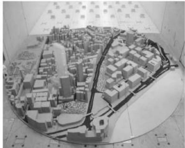
Figure 4: A design undergoing AVA Detail Study using wind tunnel.
