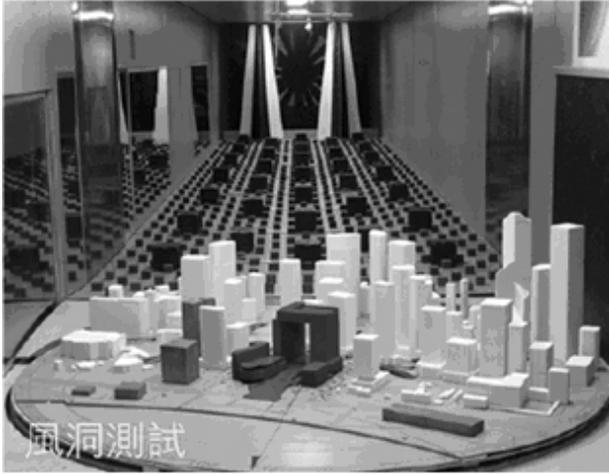
Figure 9: AVA Detail Studies using 1:400 model in a wind tunnel. (Courtesy Rocco Design Architects Ltd.)
