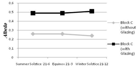
Figure 7: Impact of the glazing on the albedo of surfaces
