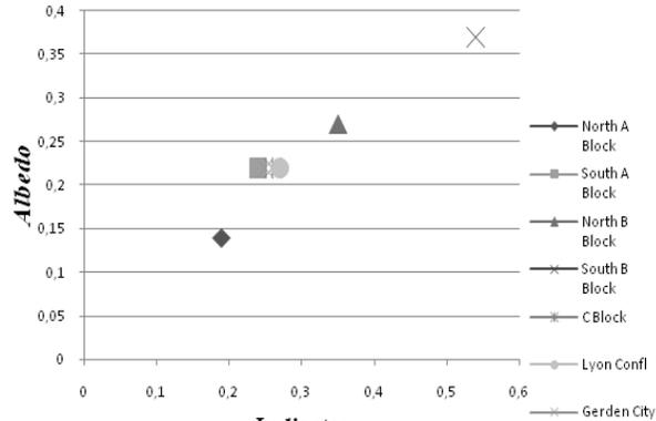
Figure 9: Comparison of A and calculated equivalent albedo for all block (summer solstice)
