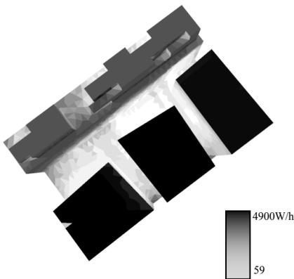
Figure 5: Energy solar absorbed, 21-3 of Block A North
