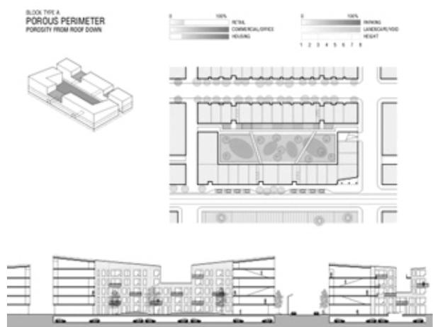
Figure 9: Diagram of mixed-use Permeable Perimeter Block
